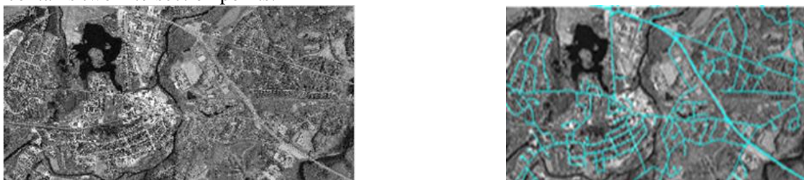
Figure.4. Road extraction based on NDVI : (a) Sample of an aerial imagery (b) Vector map of aerial imagery
